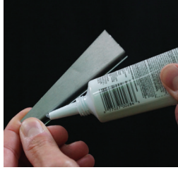
Apply a small amount of sealant down the length of the crease.
