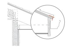
**FLASHINGS**Flashings shall be applied according to the asphalt shingle manufacturer's printed instructions. ...Base flashing R905.2.8.1,3,4 shall be of either corrosion-resistant metal of minimum nominal 0.019-inch (0.5 mm) thickness or mineral surface roll roofing weighing a minimum of 77 pounds per 100 square feet (4 kg/m2). Cap flashing shall be corrosionresistant metal of minimum nominal 0.019-inch (0.5 mm) thickness.
